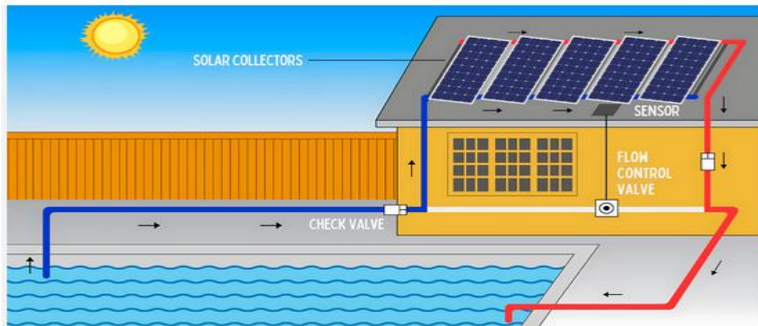
Figure 9. Swimming Pool Heating (Source: https://www.theengineeringchoice.com/what-is-solar-pool-heater/ )
